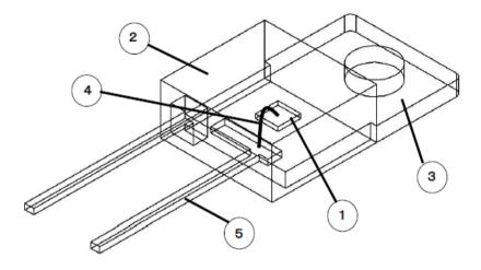
A direction of wire bonding and die bonding, a shape of frame, die size and the number of wires differ by P/N.
